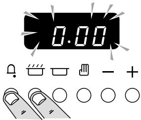
Press and hold as shown. At the same time, press (-) or (+) until the correct time shows. Don't forget it's a 24-hour clock. If you make a mistake or press the wrong button, turn off the power supply for a minute or two and start again.
