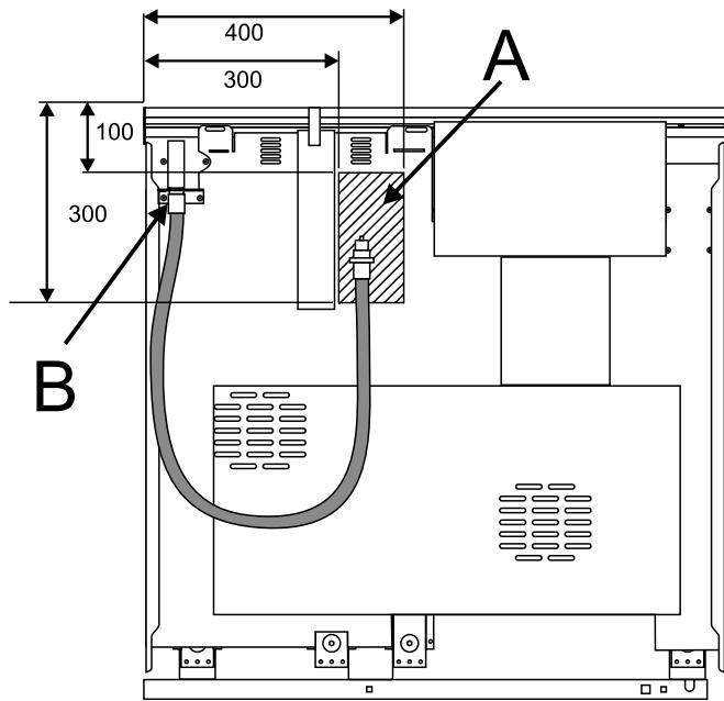
The rear cover boxes limit the position of the supply point. The house gas supply needs to terminate with a down facing connection.
