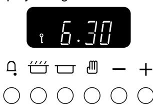
The clock oven control functions are now locked. After a few seconds the display will revert to show the time of day and the key symbol.
