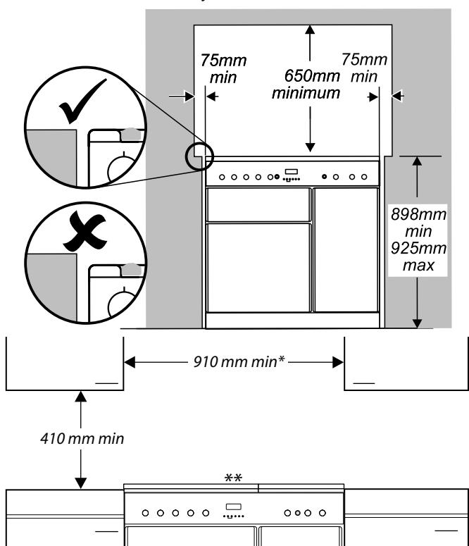
75mm should be left between each side of the cooker and any adjacent vertical surface.
