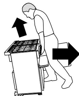
If a stability chain is fitted, release it as you ease the cooker out. Don't forget to refit it when you replace the cooker.
