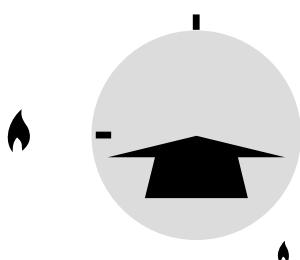
Press the igniter button or light with a match. Keep pressing the control knob in for about 10 seconds
