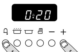
You can check time remaining by pressing [ $\text{D}.$ ] and cancel the beeper by pressing [ $\text{D}.$ ].
