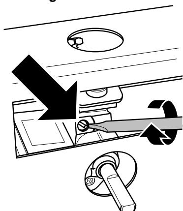
Turn the bypass screw on each control clockwise until it stops.
