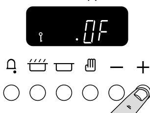
Press the '+' button once. The key symbol [!] and 'Of' shows on the display. Let go of the buttons.
